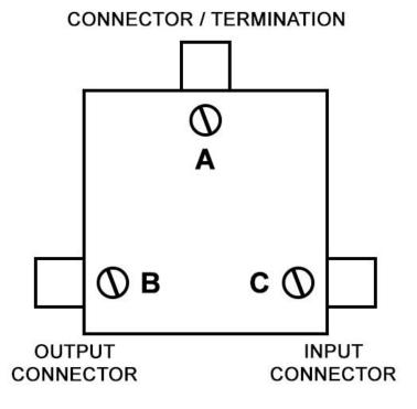
Before starting the tuning procedure please connect the termination to the correct connector (circulators only), it would be better to mount the circulator / isolator in the final place and use the definitive termination (where needed) before tuning it.
