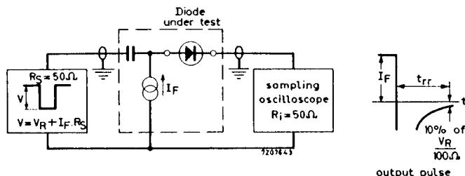
Reverse pulse: Rise time  $t_r = 0.6 \text{ ns}$ Pulse duration  $t_p = 100 \text{ ns}$ Duty cycle  $\delta = 0.05$ Circuit capacitance  $C < 1 \text{ pF}$  ( $C = \text{Oscilloscope} + \text{parasitical capacitance}$ )Recovered charge when switchedfrom  $I_F = 10 \text{ mA}$  to  $V_R = 10 \text{ V}$ ;  $R_L = 1 \text{ k}\Omega$
