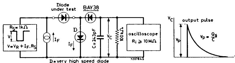
Reverse pulse: Rise time  $t_r = 2 \text{ ns}$ Pulse duration  $t_p = 0.4 \mu\text{s}$ Duty cycle  $\delta = 0.02$
