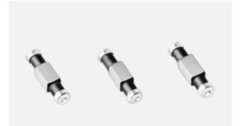
The T-type chip, NFM61R/RH, is a 3 terminal capacitor capable of carrying the large currents (2A) required for use in DC power circuits. This chip series consists of a T-type filter circuit incorporating a ferrite bead inductor for the purpose of suppressing undesirable oscillation. The heavy duty NFM61RH is an improved version of the filter for use in harsh operating conditions.
