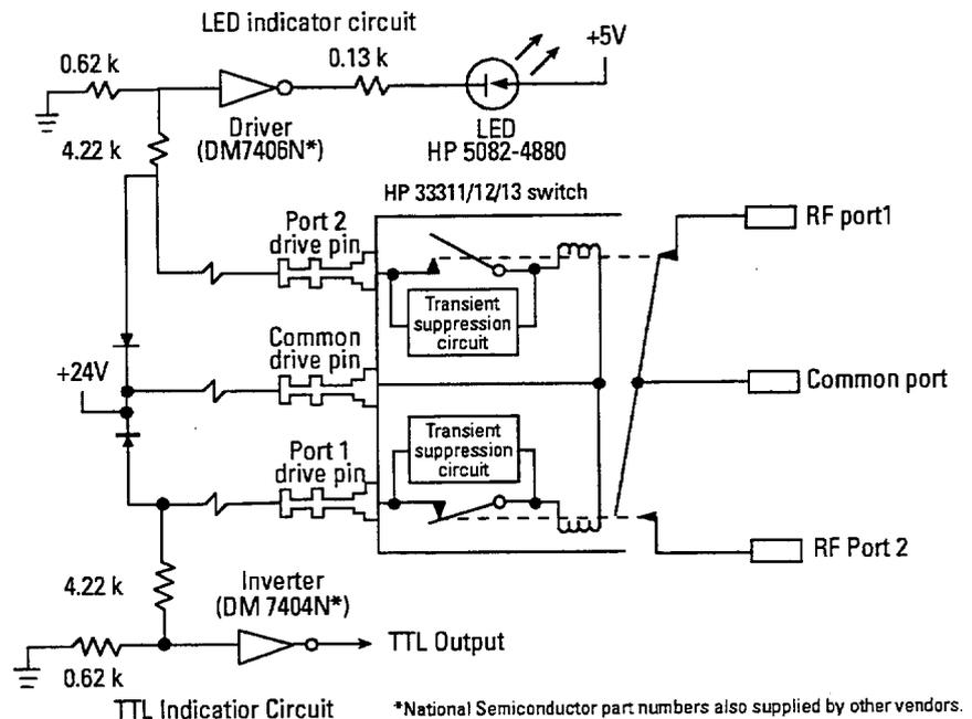
Figure 7. TTL and LED remote indicator circuits
