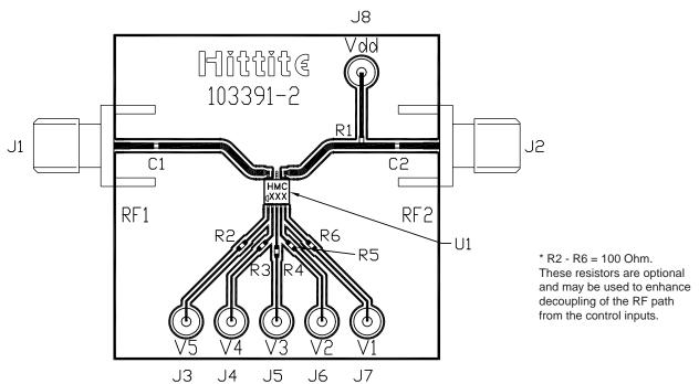
The circuit board used in the final application should use RF circuit design techniques. Signal lines should have 50 ohm impedance while the package ground leads and exposed ground paddle should be connected directly to the ground plane similar to that shown below. A sufficient number of VIA holes should be used to connect the top and bottom ground planes. The evaluation circuit board as shown is available from Hittite Microwave Corporation upon request.
