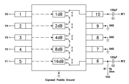
DC blocking capacitors C1 & C2 are required on RF1 & RF2. Choose C1 =  $C2 = 100 \sim 300$  pF to allow lowest customer specific frequency to pass with minimal loss. R1 = 5K Ohm is required to supply voltage to the circuit through either PIN 6 or PIN 10.
