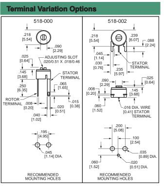
For dimensions  $\leq$  .125"/3.18mm, tolerance is ±.005/0.13 For dimensions  $\geq$  .126"/3.20mm, tolerance is ±.015/0.38
