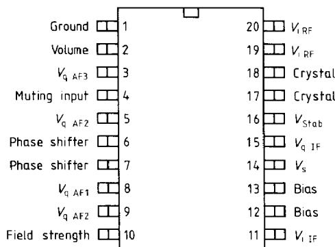
**Characteristics** $V_S = 4.5 \text{ V}$ ,  $T_A = -30^\circ\text{C}$  to  $60^\circ\text{C}$
