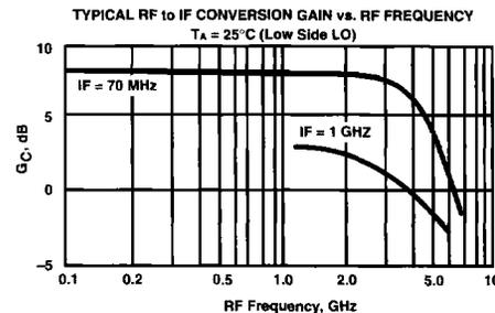
**Electrical Specifications<sup>1</sup>,  $T_A = 25^\circ\text{C}$**
