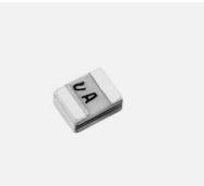
When using chip components in the design of FM radios, their arrangement and space allocation can create design difficulties. To help reduce these problems, Murata has developed this series of chip ceramic discriminators. They have heat resistant structures and allow the design of FM detecting circuits requiring no adjustment. Also, these discriminators yield stable demodulation characteristics. The CDACV10.7 Series can be used as kits with the Cerafil® SFECV10.7 Series to facilitate design.
