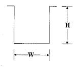
The table above indicates channel dimensions for a number of typical Supershield solid round sections. The Supershield section will provide an effective EMI seal at lower compressions, however, it will become less efficient as a pressure seal.
