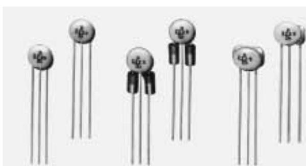
Disc-type EMIFIL® DS310, DST310 and DSS310 are T-type EMI suppression filters. The disc-type EMIFIL increases the self-resonant frequency of the capacitor by attaching two lead wires to one of the electrodes of the capacitor and increases the insertion loss by adding inductance to the lead in the DST and DSS types only. Frequencies to be suppressed can be selected by choosing the capacitance. They are also recommended for use as by-pass capacitors.
