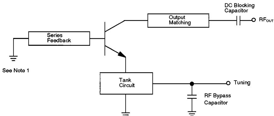
NOTE 1: DC bias lines (not shown) have internal decoupling capacitors.
