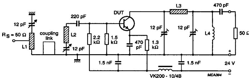
L1 = 24 mm x 6 mm x 0.5 mm silver plated copper strip. Tap of the input at 5 mm from earth.
