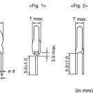
[Bulk] Vertical Crimp Short (Fig. 1) Straight Short (Fig. 2)
